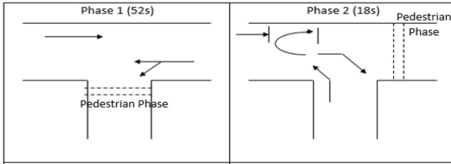
Figure 10: Phasing and timing for Scenario 3
