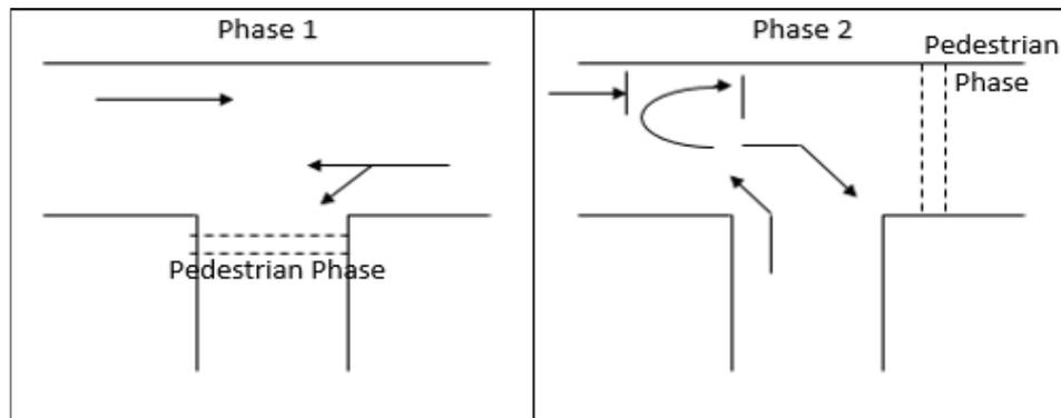
Figure 5: New phasing arrangement
