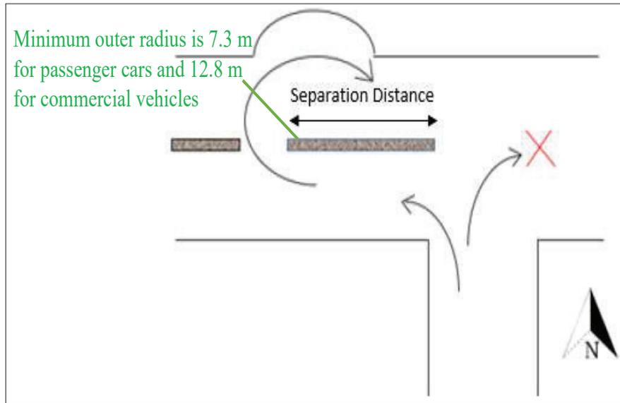
Figure 6: Separate opening with the loons provided
