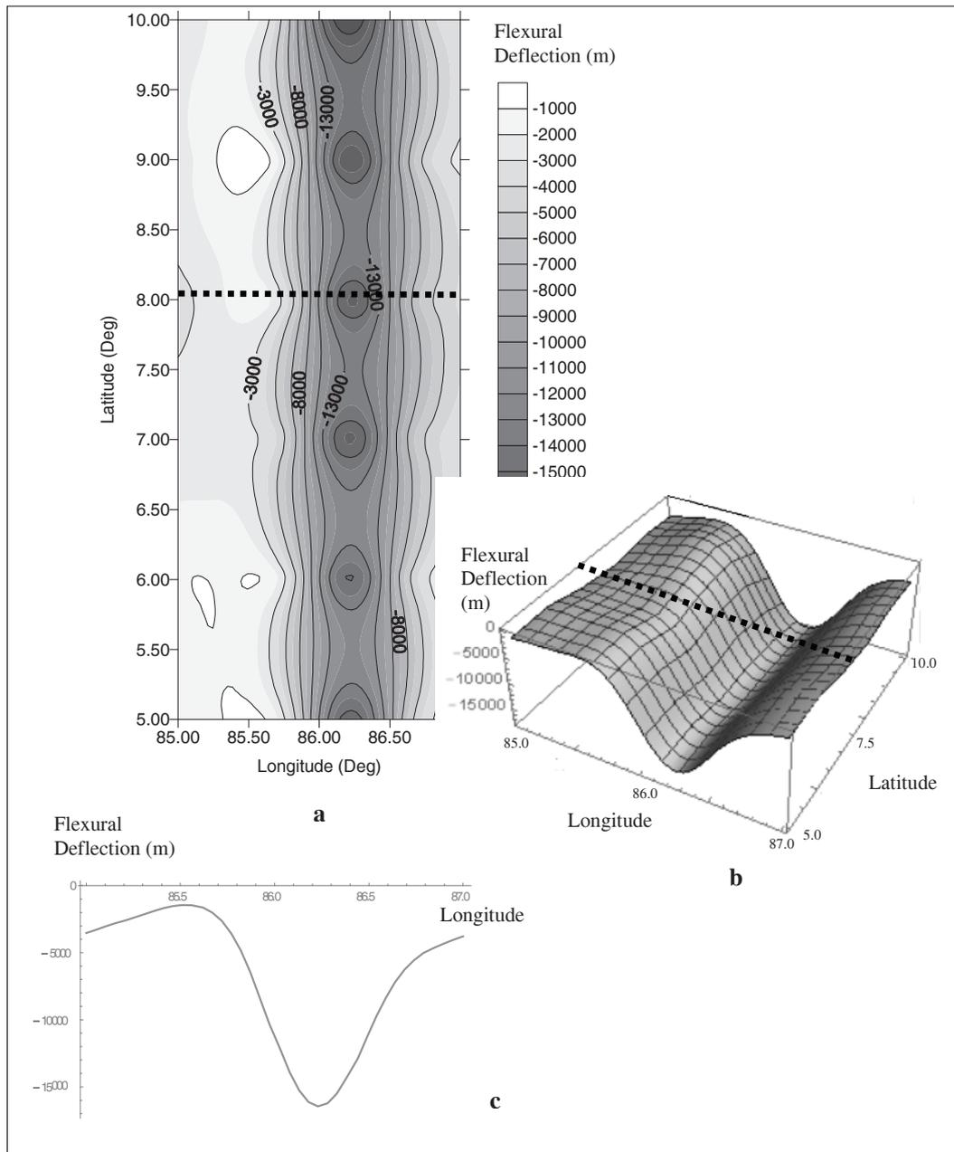
**Figure 8:** Downward deflection of oceanic crust below the 85° E ridge when flexural rigidity of the oceanic crust is  $1.8 \times 10^{21}$  Nm (a : contour map; b : 3D map and c : cross section along 8° latitude)
