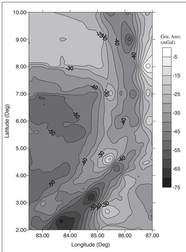
**Figure 2:** Free air gravity anomaly map over the 85° E Ridge and the surrounding area. Contours in intervals of 5 mGal
