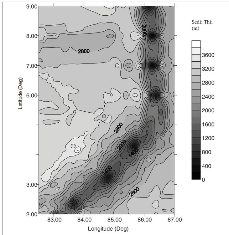
**Figure 7:** Map of sediment thickness over the 85° E ridge and the surrounding area. Contours in intervals of 200 m
