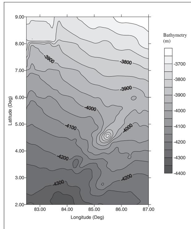
**Figure 3:** Bathymetry map over the 85° E Ridge and the surrounding area. Contours in intervals of 50 m
