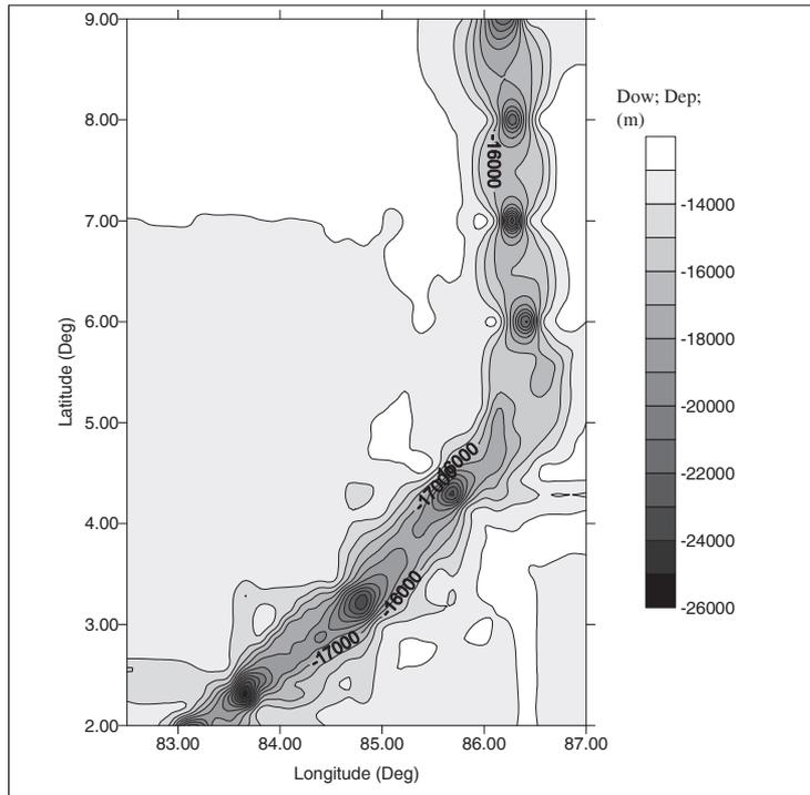
**Figure 6:** Map of downward depression of the lower layer of the oceanic crust over the 85° E ridge and the surrounding area. Contours in intervals of 1000 m
