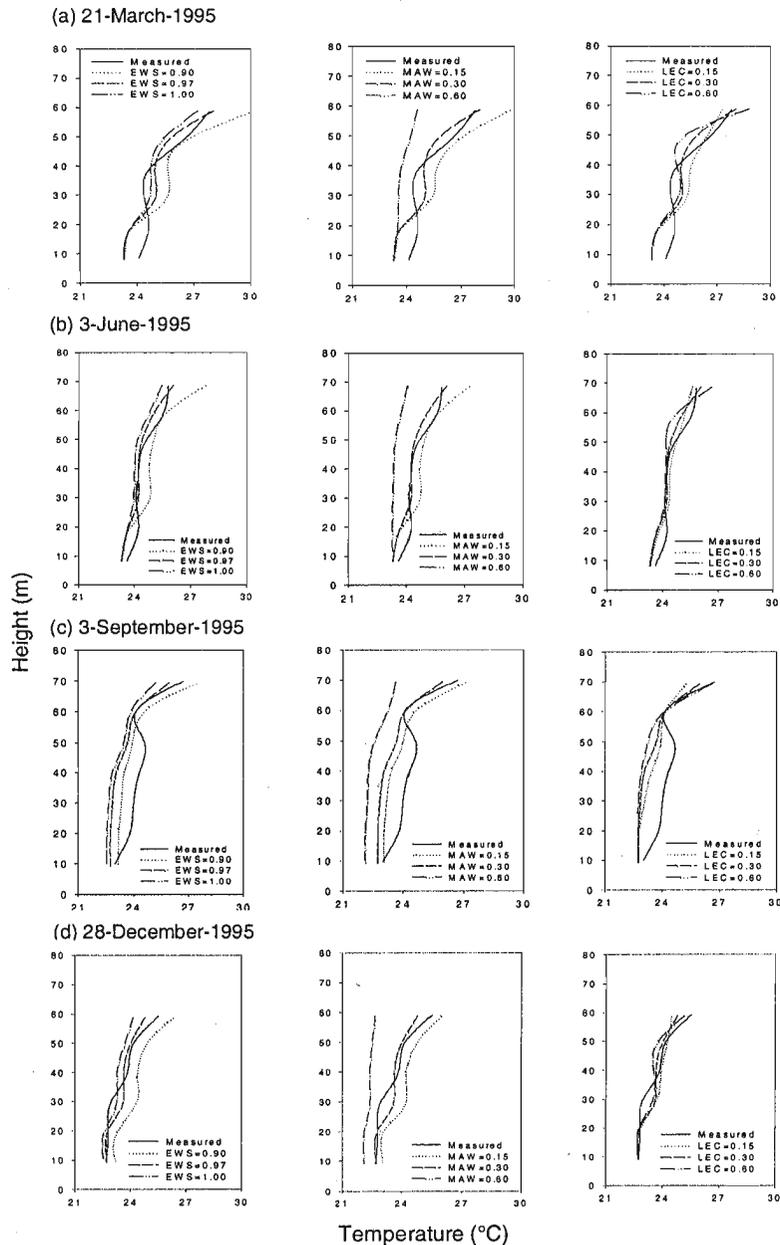
**Figure 5: Sensitivity analysis of DYRESM parameters, mean albedo of water, emissivity of a water surface and light extinction coefficient based on the temperature profiles of 21/3/1995, 3/6/1995, 25/9/1995 and 28/12/1995**
